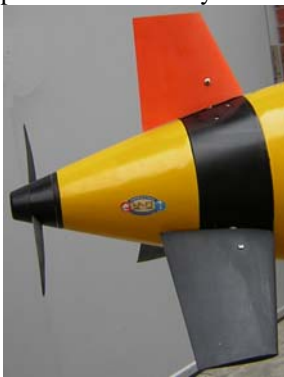
Inverted 'Y' Configured Tail Assembly
