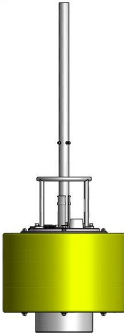
Figure 5. RF to acoustic gateway buoy.
